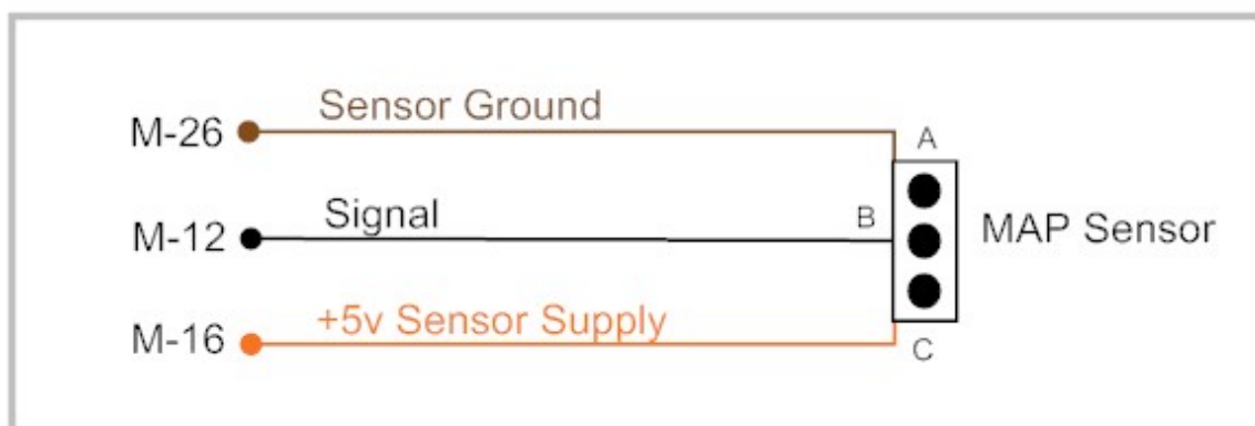
Manifold Absolute Pressure Sensor Wiring
