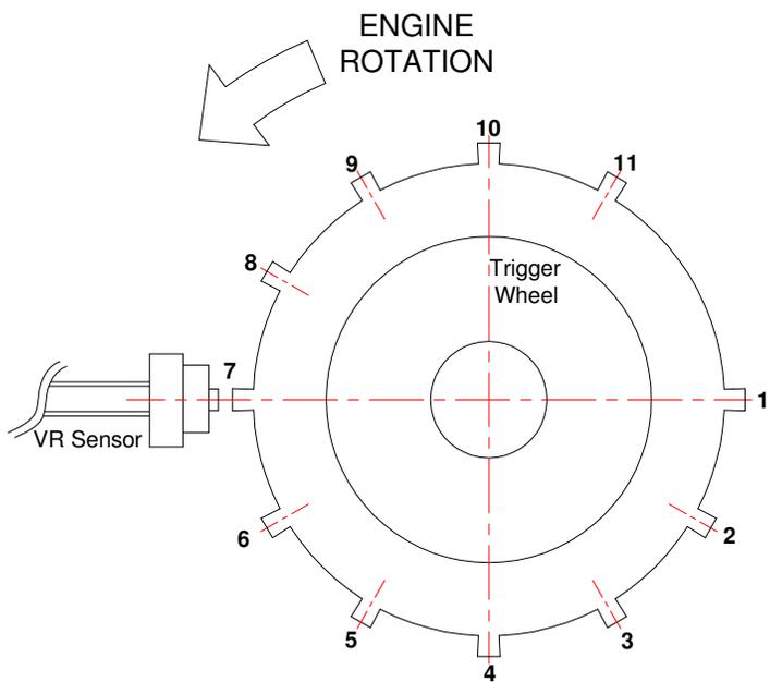
Trigger Wheel and Sensor are Shown in the Position of TDC for the Cylinder of Interest
