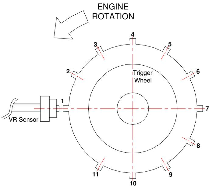
Trigger Wheel and Sensor are Shown in the Position of TDC for Cylinder #1
