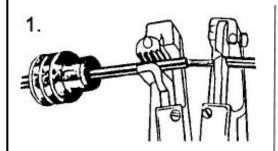
Install the seal on the cable before stripping the wire
