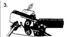
Put terminal and seal in crimping tool and and fully crimp
